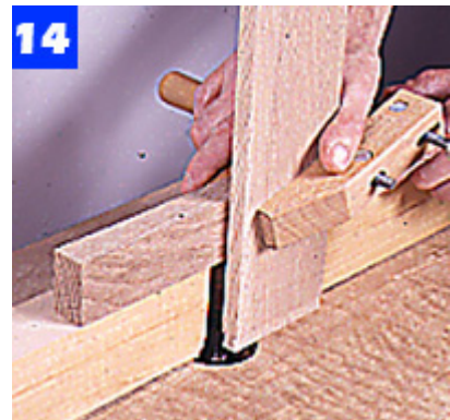
Use the same dovetail bit in a router table to cut both sides of the dovetails on the ends of each drawer side.
