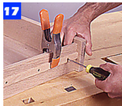
Slide the drawer bottom in place and attach it to the back with screws. Also, screw the guide strips to the sides.
