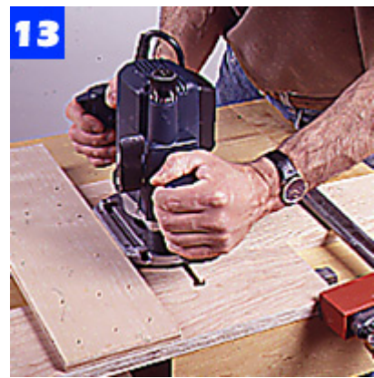
Rout slots in the drawer face for the drawer sides with a dovetail bit. Use a square U-shaped jig to guide the router.
