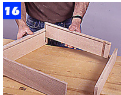
Apply glue to all the drawer joints, then clamp the box together. Reinforce the side-to-back joints with brads.
