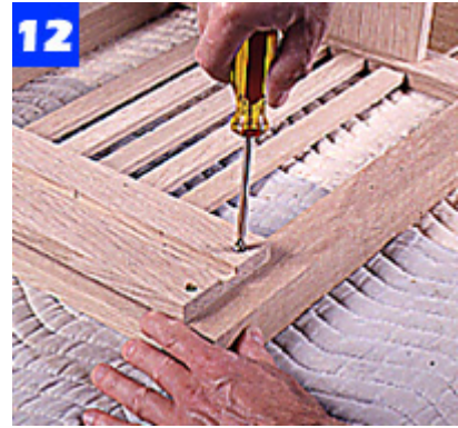
Bore and countersink pilot holes in the drawer guide strips. Then attach them to the legs with 1-1/4-in. No. 8 fh screws.
